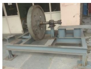
Figure 29. Flywheel – shaft - bearing mounted on frame with drive motor &amp; generator mount
