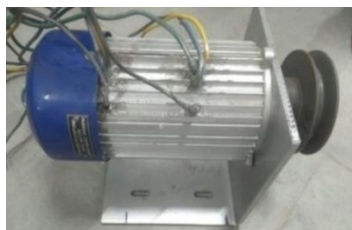
Figure 20. Drive motor with motor mount & drive pulley
