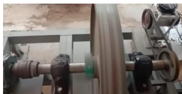
Figure 22. Driver & driven pulley, belt arrangement, flywheel mounted on shaft, 2 cylindrical roller bearings & jaw coupling
