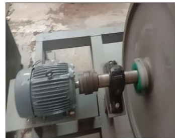
Figure 27. Flywheel Connected to Generator via Jaw Coupling supported by Bearing
