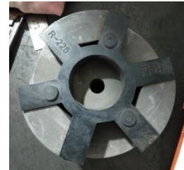
Figure 25. Jaw coupling with rubber bush in between
