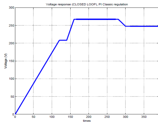
Figure 11. Voltage across the armature
